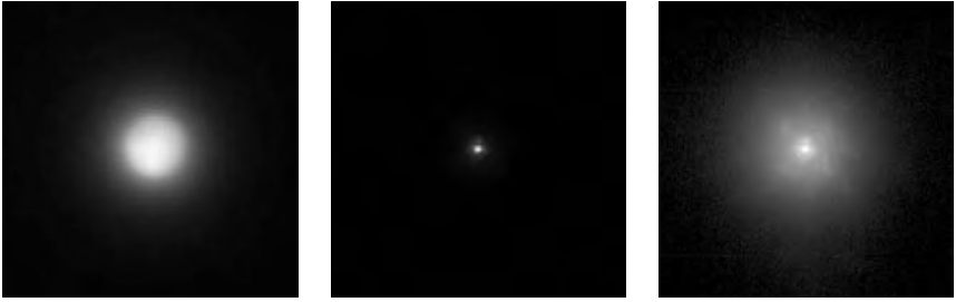
Figure 4.7. Left, the observed image; center, the instrument response (IR) on a linear scale; and right, the logarithm of this response thresholded at 1/1,000th of its maximum. On the IR, a central peak can be observed, with a vast plateau spreading over most of the image support
