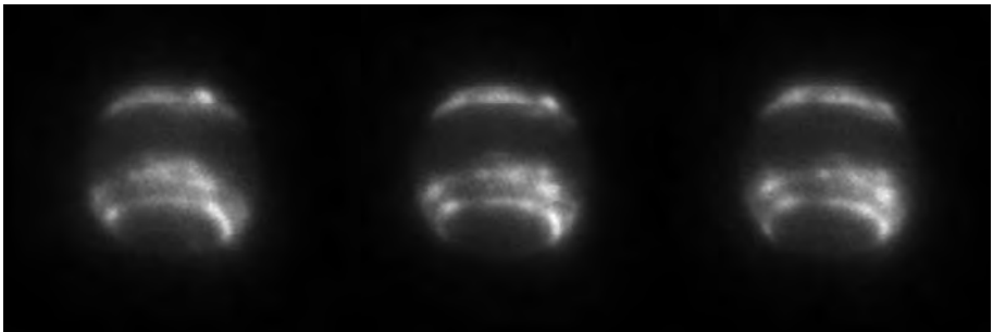
Figure 10.9. Images of Neptune obtained at 30-minute intervals on 6th July 1998 with the Hokupa'a adaptive optics system on the Canada-France-Hawaii telescope. The imaging wavelength was 1.72\ \mu\text{m} and the exposure time for each image was 10 minutes
